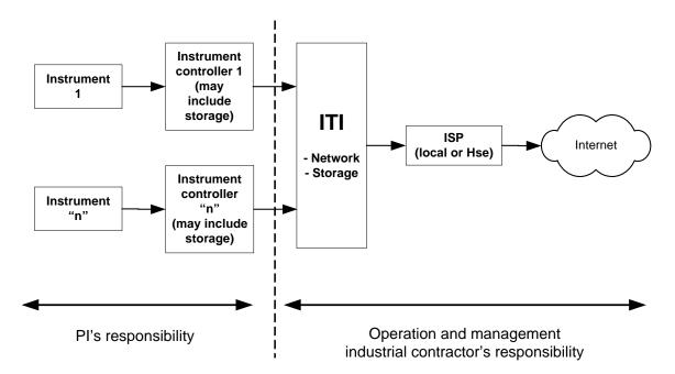
The IT infrastructure provides basic network services, shared storage, and serial data acquisition capabilities at each GO core site. It is capable of autonomous operation under non-ideal conditions such as dusty environments, poor power quality, and potentially extreme temperatures.
