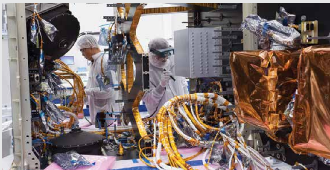
Engineers inspect the second of three RCM satellite buses in the Magellan facility. Batteries are visible in the foreground, wrapped in thermal blankets. A reaction wheel is on the left. (2016-02-11)
